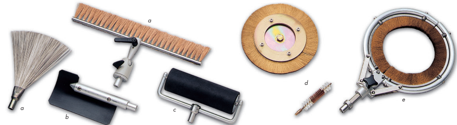
Overview of the various electrodes: a) Sweeper electrode b) Flat electrode c) Roller electrode d) Rotating electrodes for tests inside pipes e) Circular ring electrode for tests on the outside walls of pipes
