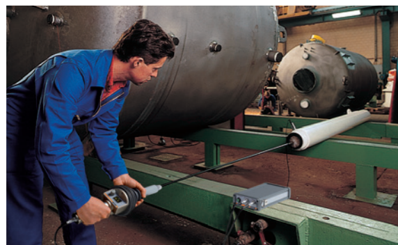
Testing the interior coating of a pipe with the POROSCOPE®, using a rotating electrode on a rod extension system
